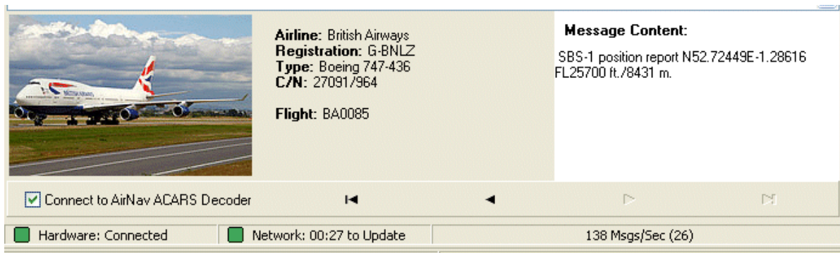
Above: ACARS aircraft and message information displayed in the RadarBox interface
